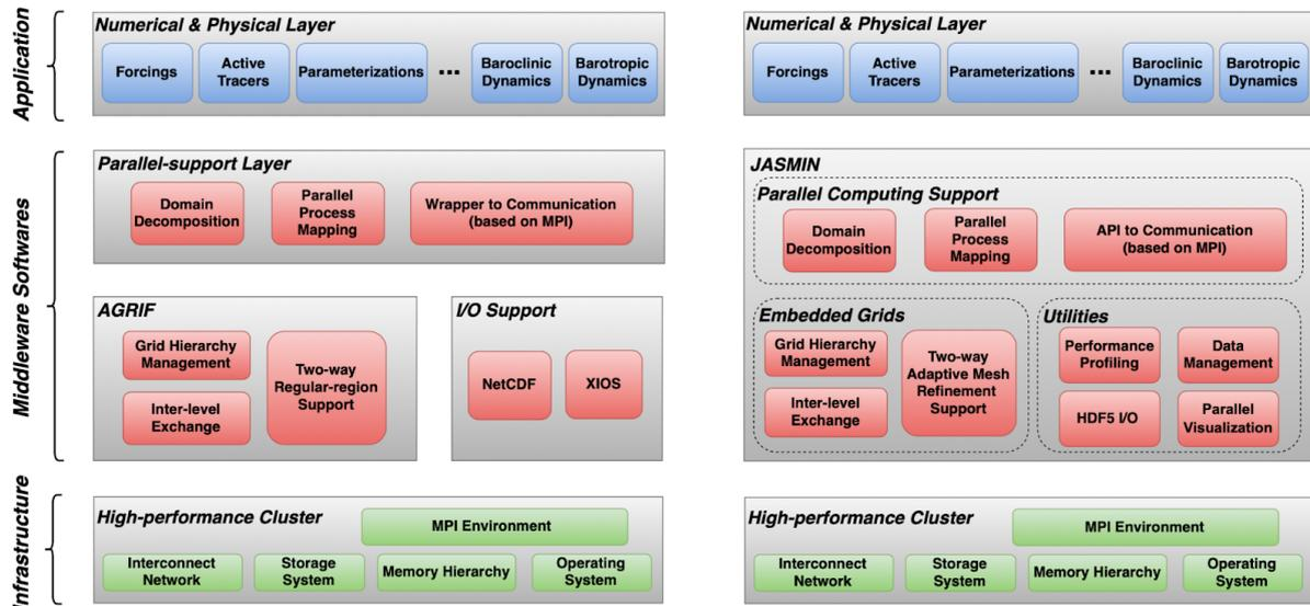
Figure 1. Model structure and abstraction layers of NEMO (left) and OMARE (right).
