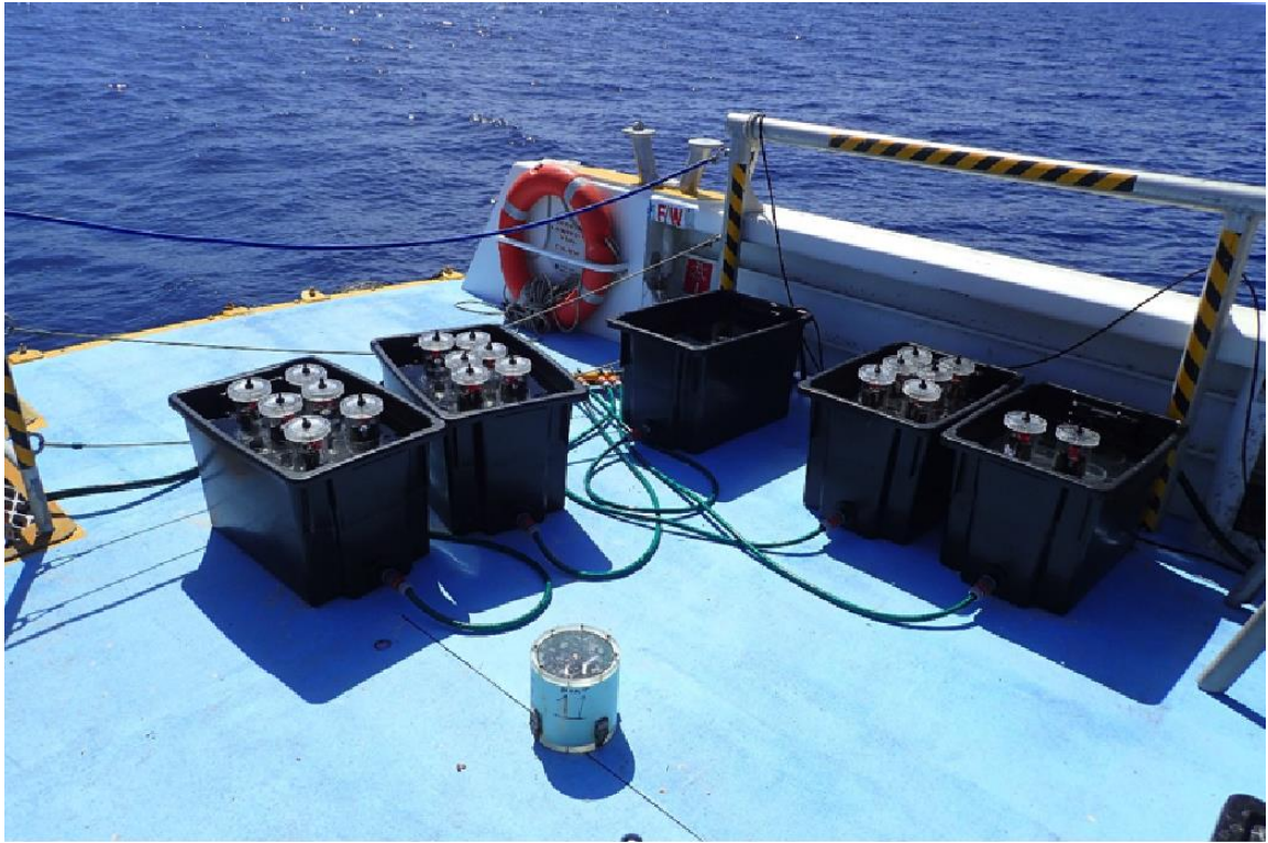
Figure 2. Experimental setup of respirometry incubations for Browse Island coral and macroalgae.
