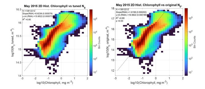
The Chl to PSD parameters bivariate histograms are shown above. They illustrate that while a relationship obviously exists (with relatively high linear R<sup>2</sup> of about 0.8), substantial variability of the PSD parameters exists for a single value of Chl, especially so for the PSD slope. This illustrates that the PSD parameters and Chl are not "one and the same thing", and we do not advocate for juts retrieving the PSD via Chl. See also Brewin et al. (2012), their Fig. 6.
