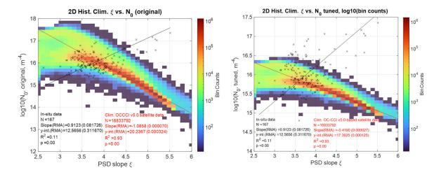
When only a few outliers are removed, the in-situ data exhibit no significant linear relationship (slope 95% confidence interval crosses zero,  $R^2 << 0.01$ ) between the two PSD parameters. See the figure below with outliers removed. We conclude that the subset of in-situ data matched with satellite data do not exhibit a significant relationship between x and N0, much unlike the satellite data, which do exhibit a strong negative correlation.
