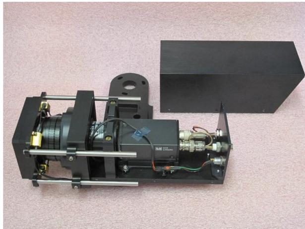
**Figure 1.** Photograph of one of the intensified video cameras equipped with a grating. The protective cover is removed and visible in the back. Power resistors to heat the grating can be seen on the left.
