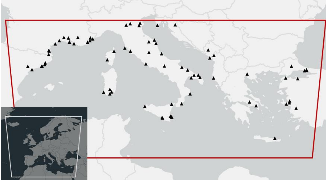
Figure 1: Domains and measurement stations. Red trapeze displays the 12 x 12 km 2 domain, black triangles are locations of measurement stations. On bottom left the larger 36 x 36 km 2 domain is displayed.
