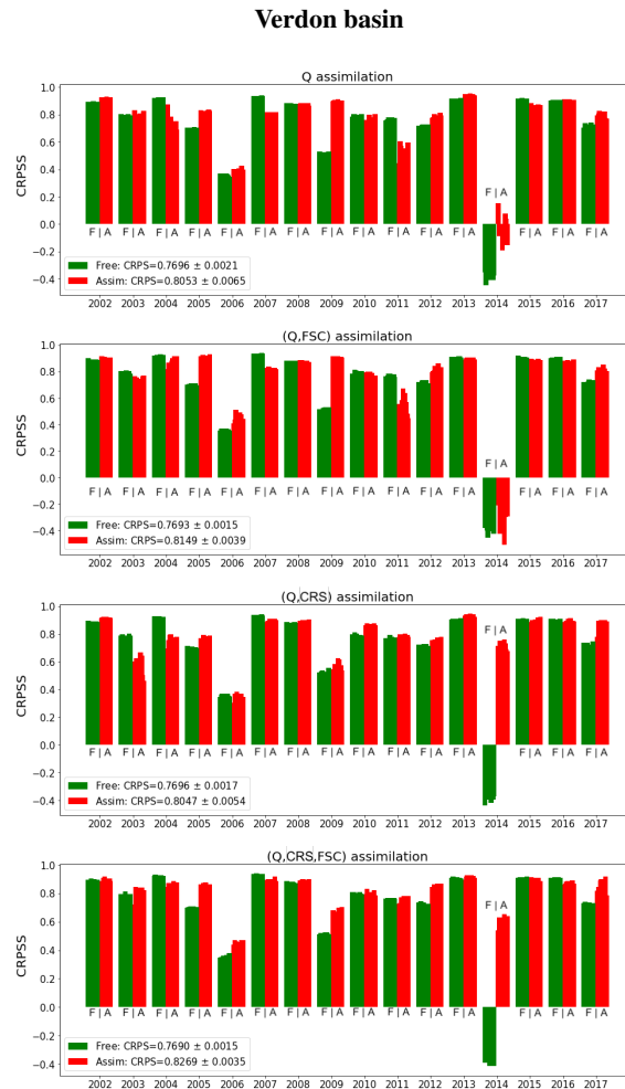
Figure 13. Yearly CRPSS of the seasonal streamflow supply SSS for the free ensemble (green) and the assimilated ensemble (red) from the Q assimilation, (Q,FSC) assimilation, (Q,CRS) assimilation and (Q,CRS,FSC) assimilation (10 experiments each year) in the Verdon basin.
