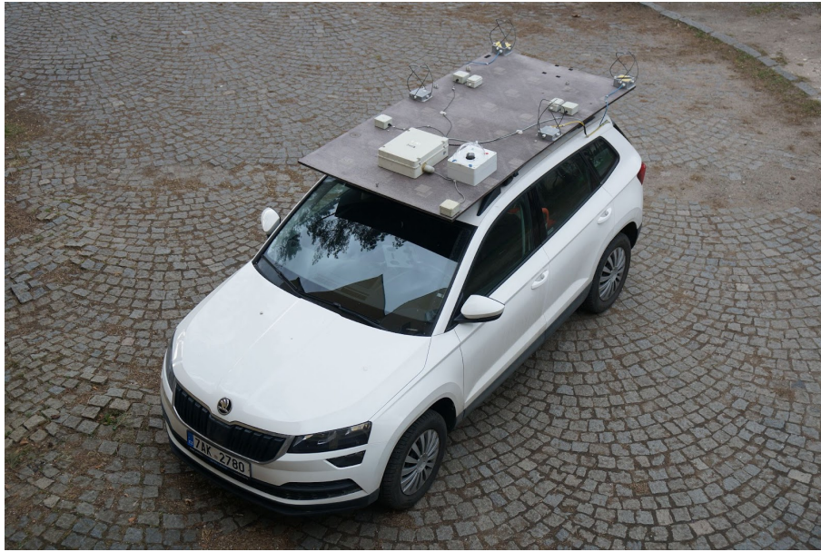
Figure 1. Measuring CAR0 with instruments mounted on the roof platform.
