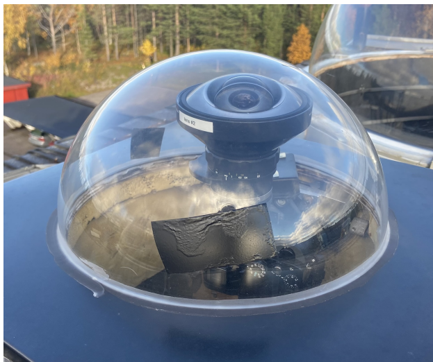
Figure 3. All-sky camera (ASC) at Swedish Institute of Space Physics in Kiruna ( 68^\circ north).
