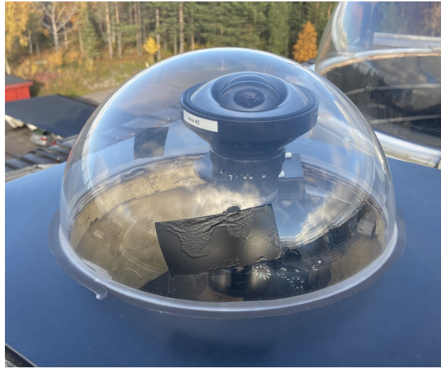
Figure 3. All-sky camera (ASC) at Swedish Institute of Space Physics in Kiruna (68° north).
