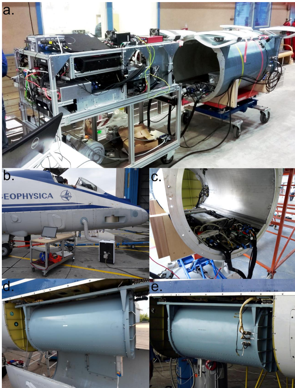
Figure S6 - Photographs from the ERICA deployment in the field: (a) the instrument and the Pressure Vessel (PV) in the hangar before installation, (b) the M-55 Geophysica at the apron with an air-conditioning unit attached to Bay II providing cooling to the ERICA, (c) close-up of the equipment installed at the bottom of the PV, (d) the ERICA installed on the aircraft as seen from the starboard side, the coiled-wire vibration isolators can be seen at the top and the removed cowl at the bottom of the photograph, and (e) the ERICA installed on the aircraft as seen from the port side, the electrical connections to the aircraft can be seen on the RHS of the photograph.
