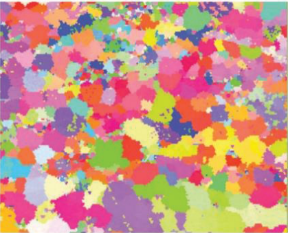
Figure C1: Electron backscatter diffraction (EBSD) map showing the orientation of quartz C-axis in layer
