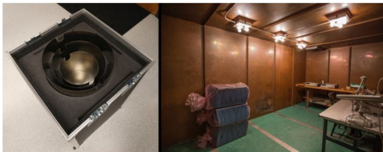
Figure 6. Zero Gauss Chamber (left) and Copper Room (right) used for Resolution Test (from Regoli et al. (2018b))
