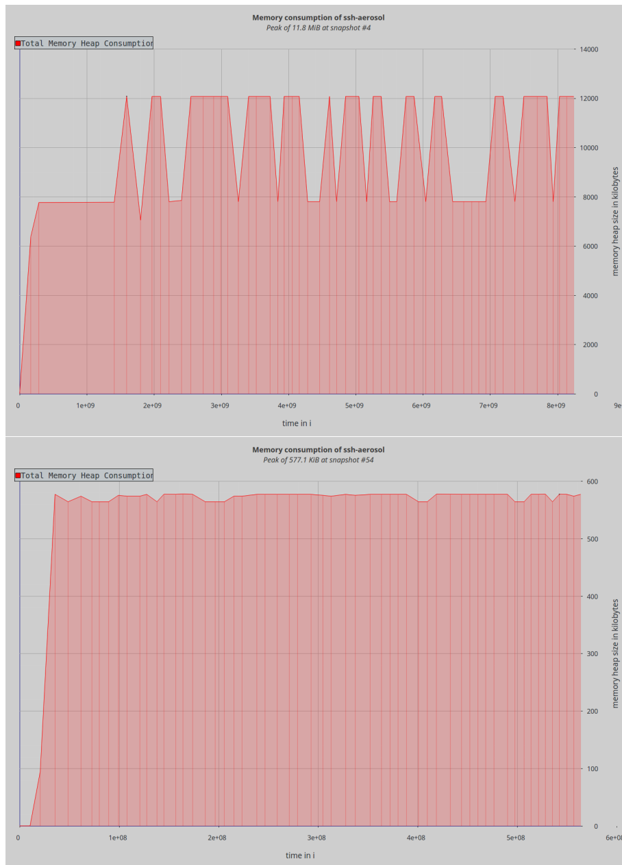
Figure 1: Memory maps for MCM (top panel) and "Rdc." (bottom panel) mechanisms simulated with SSH-aerosol under the same conditions. The graphs are generated with massif-visualizer.
