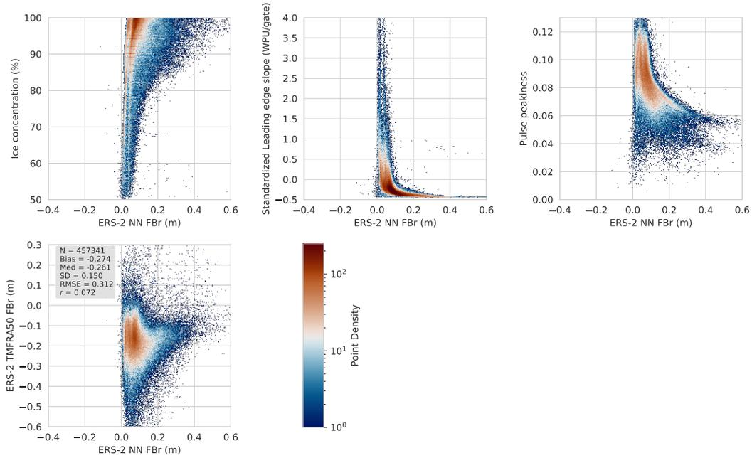
**Figure A3.** An outline of the link established by the NN between some of the inputs (Standardized LES, PP, sea ice concentration and TFMRA50 FBr) and ERS-2 NN FBr. WPU means Waveform power unit, for ERS-2 correction
