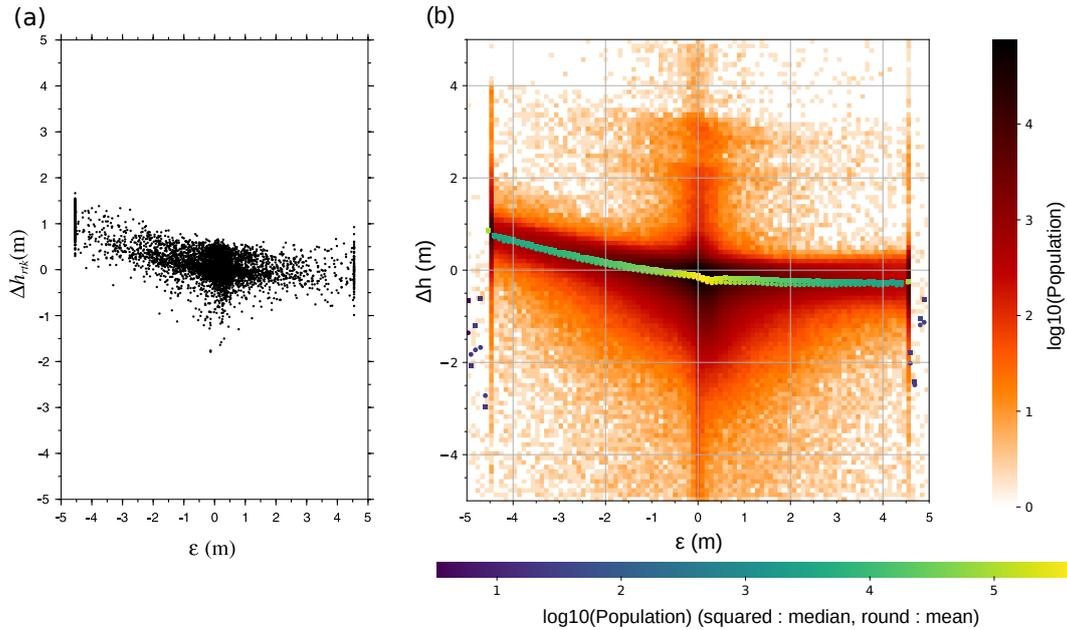
**Figure 3.** Difference between the raw surface measurements and the interpolated ocean level measurements as a function of the height error parameter  $\epsilon$ . (a) is taking from Peacock and Laxon (2004) and (b) a reproduction for the Cycle 83 of ERS-2. On (b) squares and circles are respectively the median and the mean of  $\Delta h$  for each value of  $\epsilon$  (on the x-axis).
