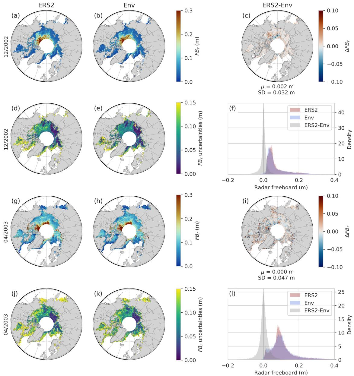
**Figure 8.** Same as Figure 7 but for ERS-2 and Envisat during December 2002 and April 2003. Histograms only include data for the coinciding region between ERS-2 and Envisat.  $\mu$  refers to the mean difference and  $SD$  to the Standard Deviation of the difference.
