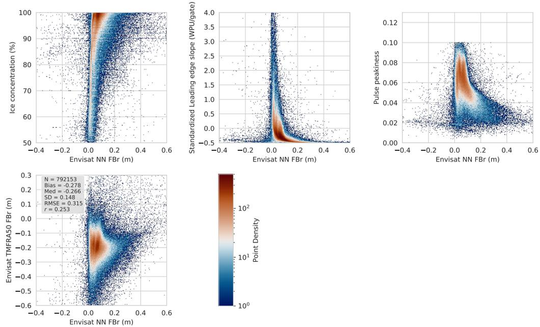
**Figure A2.** An outline of the link established by the NN between some of the inputs (Standardized LES, PP, sea ice concentration and TFMRA50 FBr) and Envisat NN FBr. WPU means Waveform power unit, for Envisat correction.
