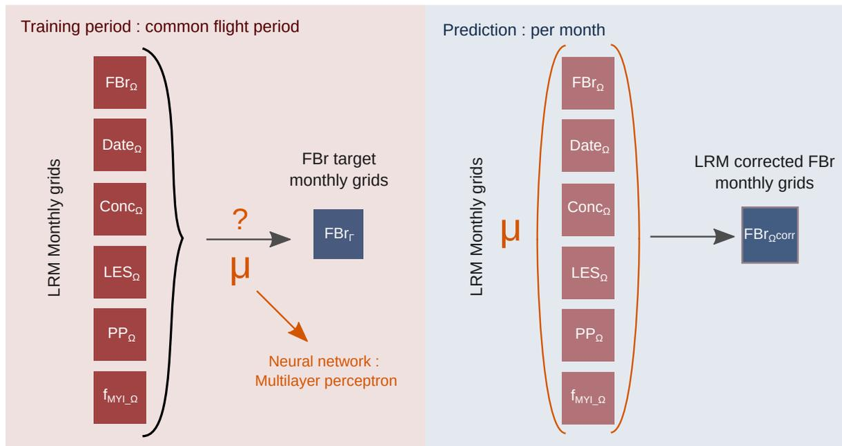
**Figure 5.** Diagram illustrating the principle of freeboard correction by neural network with the two main steps: on the left panel, the neural network training phase, and on the right panel, the prediction (correction) phase.  $\Omega$  corresponds to the inputs and  $\Gamma$  the output of the Neural Network. FB: radar freeboard, Conc : Sea ice concentration, LES: Leading Edge Slope, PP, Pulse Peakiness,  $f_{MYI}$ , MYI proportion.
