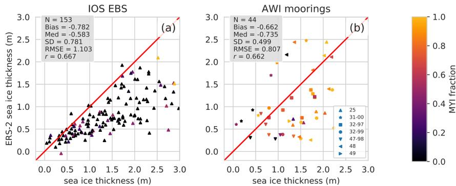
**Figure 12.** Comparative scatter-plots between ERS-2 NN sea ice thickness estimations and 2 anchored moorings data sets. The x-axis shows sea ice thickness estimations from (a) IOS Beaufort Sea and (b) AWI moorings sea ice draft. The color bar indicates the respective MYI proportion.  $N$  is the number of the couple of values that are compared, Med refers to the Median, SD the Standard deviation, RMSE the Root Mean Square Error and  $r$  the correlation coefficient.
