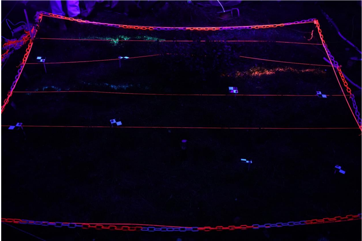
Figure S7: Nighttime photo of the 1860M plot, taken after the high intensity (HI) experiment. The sand was illuminated with two LED lamps before and with six UV lamps before and while taking the photo. The orange sand ribbon was added prior to the low intensity experiments (LI), the green sand prior to the medium intensity (MI) experiments, and the blue sand prior to the HI experiments.
