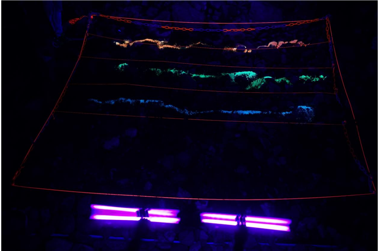
Figure S10: Nighttime photo of the 1990H plot, taken after the high intensity (HI) experiment. The sand was illuminated with two LED lamps before and with six UV lamps (of which two can be seen at the bottom of the photo) before and while taking the photo. The orange sand ribbon was added prior to the low intensity experiments (LI), the green sand prior to the medium intensity (MI) experiments, and the blue sand prior to the HI experiments.
