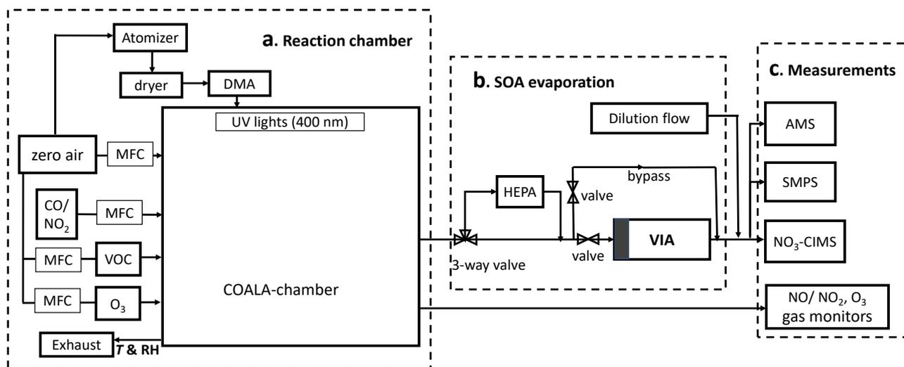
**Figure 1. Setup for the thermal evaporation experiments used in this work. Note that all three parts (a, b, and c) are necessary for the particle-phase HOM measurements, whereas only part a and c are used for the gas-phase HOM measurements (i.e. all instruments sampling directly from the chamber).**
