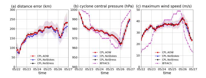
**Figure A4.** The characteristics of cyclone Mekunu obtained from the coupled simulations that do not consider the effect of Stokes forces (Stokes-Advection and Stokes-Coriolis) and wind stress corrections. The solid lines indicate the ensemble averaged simulation results; the shaded areas indicate the standard deviation of the results. Panel (a) shows the distance errors in comparison with IBTrACS data; Panel (b) shows the cyclone central pressure; Panel (c) shows the maximum wind speed.
