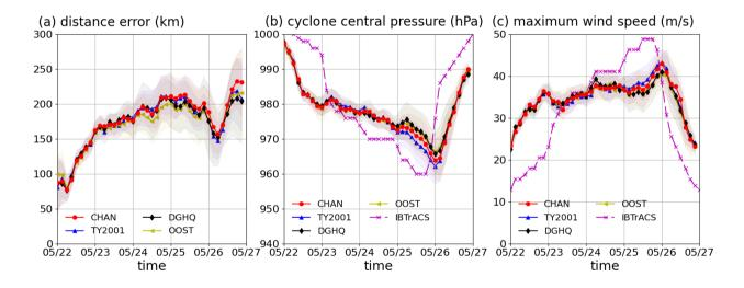
**Figure A3.** The characteristics of cyclone Mekunu obtained from the coupled simulations using different options to parameterize surface roughness. The solid lines indicate the ensemble averaged simulation results; the shaded areas indicate the standard deviation of the results. Panel (a) shows the distance errors in comparison with IBTrACS data; Panel (b) shows the cyclone central pressure; Panel (c) shows the maximum wind speed.
