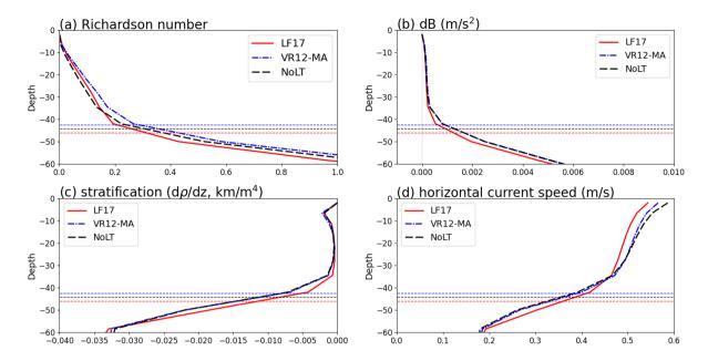
**Figure 11.** The snapshots of the vertical profiles at 00 UTC May 24 obtained in the simulations. Panel (a-d) show the Richardson number, buoyancy term, density changes, and horizontal velocity. The solid lines indicate the vertical profiles obtained from CPL.NoLT, CPL.VR12-MA, and CPL.LF17. The horizontal dashed lines indicate the mixed-KPP boundary layer depth in MITgcmto illustrate the mixing layer.
