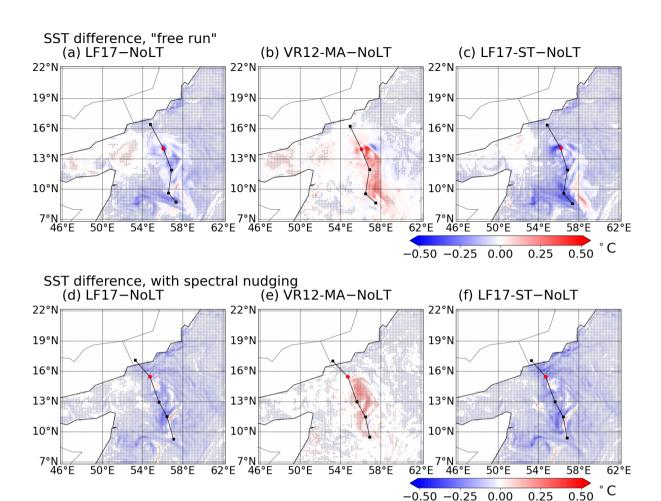
**Figure 9.** The snapshot snapshot of the ensemble averaged SST difference. Panels (a-c) show the SST difference between the simulations with Langmuir turbulence (CPL.LF17, CPL.VR12-MA, and CPL.LF17-ST) and without Langmuir turbulence (CPL.NoLT). Panels (d-f) show the same differences in the simulations with spectral nudging. The markers indicate the regions where the SST difference is significant (P < 0.05).
