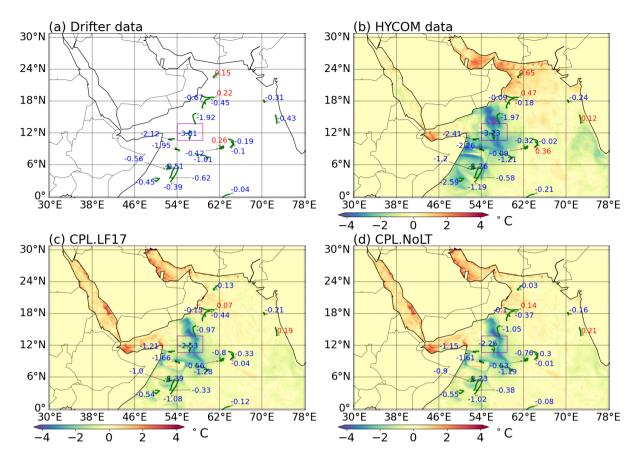
**Figure 8.** Evolution of the SST during the tropical cyclone event in comparison with drifter data. Panel (a) shows the SST changes during the event from drifter data; Panels (b-d) show the ensemble averaged SST changes from HYCOM, CPL.LF17, and CPL.NoLT, respectively. The red numbers indicate SST warming during the event; the blue numbers indicate SST cooling during the event.
