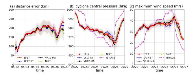
**Figure A2.** The characteristics of cyclone Mekunu obtained from the coupled simulations using different options to parameterize Langmuir turbulence. The solid lines indicate the ensemble averaged simulation results; the shaded areas indicate the standard deviation of the results. Panel (a) shows the distance errors in comparison with IBTrACS data; Panel (b) shows the cyclone central pressure; Panel (c) shows the maximum wind speed.
