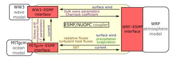
**Figure 1.** The schematic description of the SKRIPS regional coupled ocean–atmosphere model. The yellow block is the ESMF/NUOPC coupler; the white blocks are the ocean and atmosphere components; the red blocks are the implemented MITgcm–ESMF, WRF–ESMF, and WW3–ESMF interfaces.
