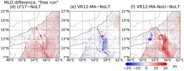
**Figure A6.** The snapshot of the ensemble averaged SST and MLD difference. Panels (a-b) show the SST difference between the simulations with Langmuir turbulence (CPL.LF17, CPL.VR12-MA) and without Langmuir turbulence (CPL.NoLT). Panel (c) shows the SST difference using VR12-MA but does not enhance the diffusion coefficient for current velocity. Panels (d-f) show the differences in MLD. The markers indicate the regions where the SST difference is significant (P < 0.05).
