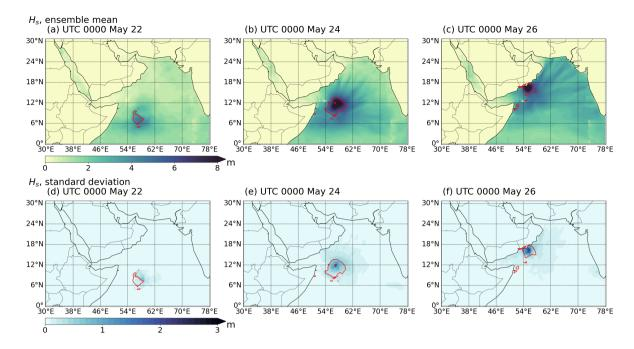
Figure 7. Snapshot Snapshot of the significant wave height  $H_s$  at 00 UTC May 22 24, and 26, 2018. Panel (aa-c) shows show the ensemble averaged  $H_s$  obtained from CPL.AOW; Panel (bd-f) shows show the standard deviation of  $H_s$  of the ensembles from CPL.AOW. The 15 m/s contour of wind speed is used to highlight the location of the tropical cyclone.
