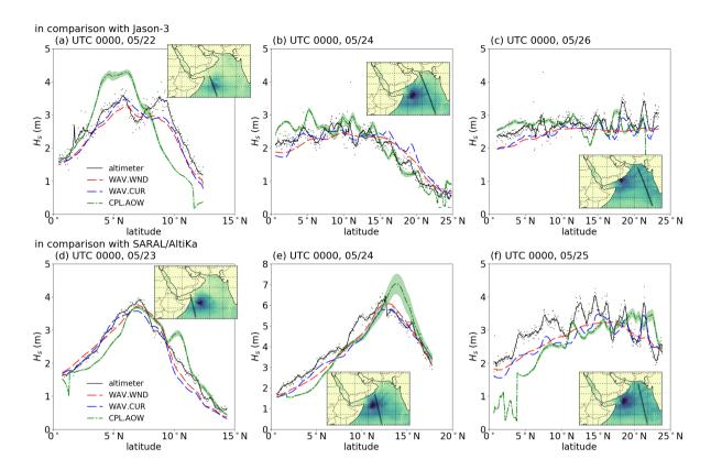
**Figure A7.** The ensemble averaged significant wave height in comparison with the altimeter data. Panels (a-c) show the comparison with Jason-3 data; Panels (d-f) show the comparison with SARAL data. The simulation results from Sun et al. (2022) are also presented. The shaded areas indicate the standard deviation of wave height in the ensemble simulations.
