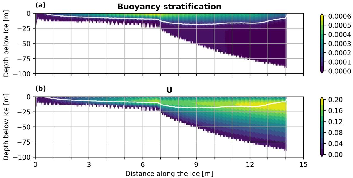
Fig. 2: Section of buoyancy (a) and along ice velocity (b) within the plume region, as defined by the horizontal velocity criterion ( $u > 0$ ). The white lines indicate the 75th percentile buoyancy isoline.
