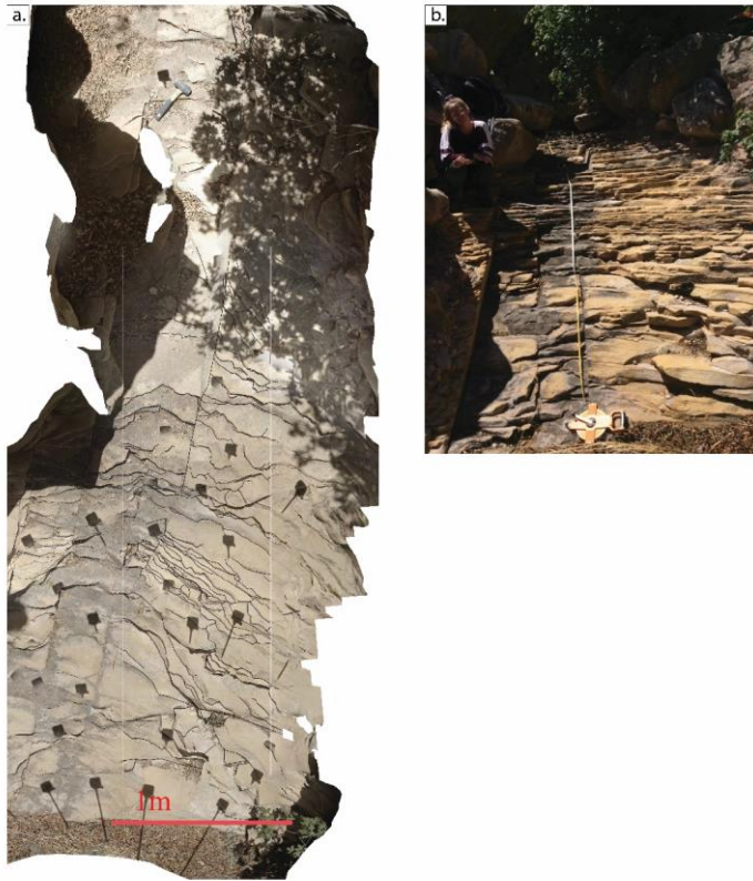
Figure 4: a) An orthomosaic and b) photo of sandstone reach LC3.2 (Figure 2b), with a discontinuity intensity of 13.03 1/m in the steep channel section. The shadows in the orthomosaic are from the GoPro and selfie stick used to film the reach. Lat, Long: 32.252513, -104.701289
