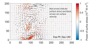
Exp-PF has produced counter currents similar to those in Exp-PD, which are set up by the Ekman pumping as described in Lines 263-267.
