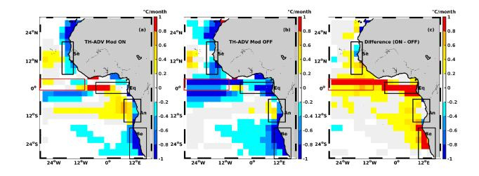
Figure R1.2: Mean horizontal heat advection from model: online re-sampled at 2.5° resolution (a), offline (b) and their difference (c). The black rectangles correspond to the 4 regions of study. The red rectangle represents the TIWs box as used in Tuchen et al. (2022).
