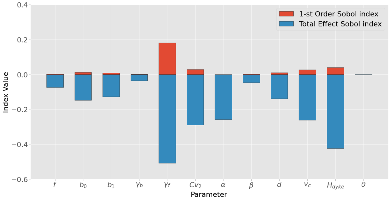
Figure 7. Value of the 1st-order sensitivity (in red) and total effect (in blue) indices for each tested parameter.
