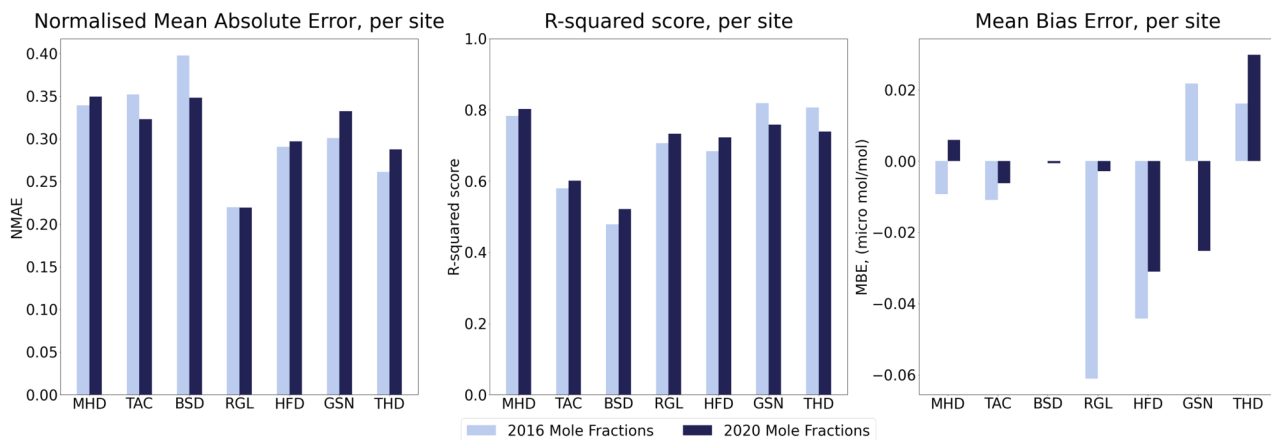
Figure 5. Evaluation of emulators with mole fraction comparison, using metrics NMAE, R-squared score and MBE, shown per site and year.
