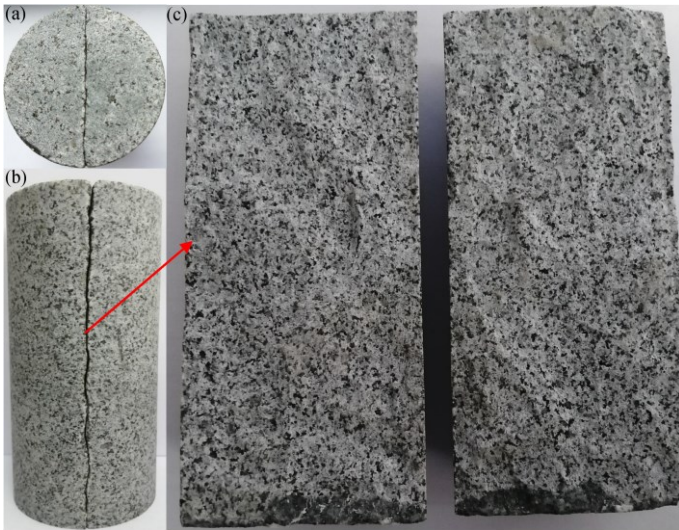
235 Fig. 9 Photo of fractured granite specimen. (a) End of specimen. (b) Side of specimen. (c) Fracture surface.
