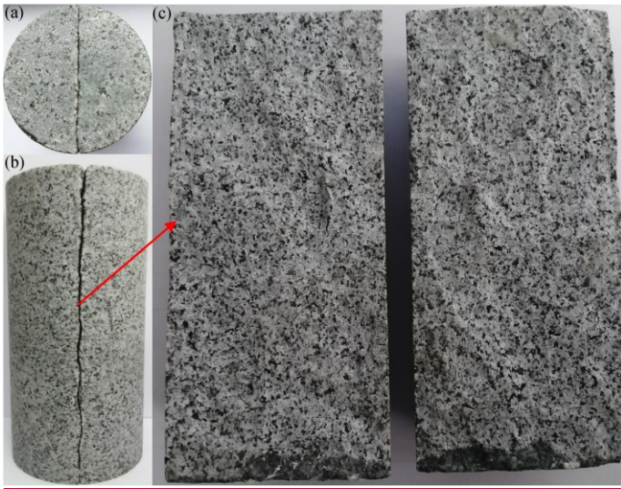
Fig. 9 Photo of fractured granite specimen. (a) End of specimen. (b) Side of specimen. (c) Fracture surface.
