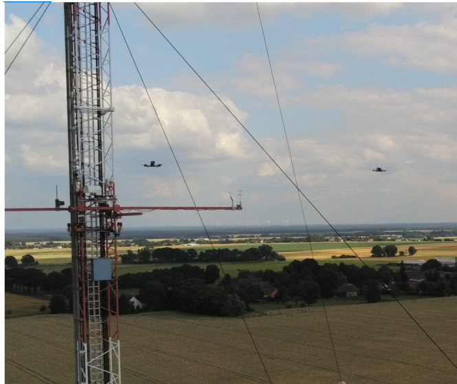
Figure 1. Two Holybro QAV250 UAS in flight. In the background the 99-m mast with a sonic anemometer on the boom at 50 m can be seen.
