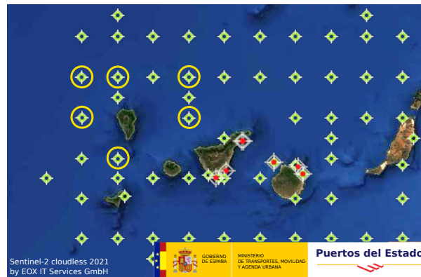
Figure 7. Set of SIMAR model points around the island, indicating the ones selected to extract the Significant Wave Height (SWH) around La Palma. Dataset downloaded from Puertos del Estado (2022) website. Map: Sentinel-2 cloudless 2021 by EOX IT Services GmbH.
