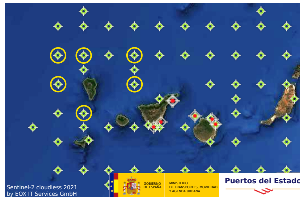
Figure 7. Set of SIMAR model points around the island, indicating the ones selected to extract the Significant Wave Height (SWH) around La Palma. Dataset downloaded from Puertos del Estado (2022) Puertos del Estado (2022) website. Map: Sentinel-2 cloudless 2021 by EOX IT Services GmbH.
